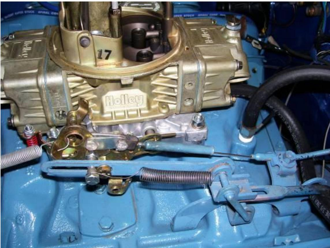
“The carb and coil detail shows what happens you put a Holley dual feed on a big block. The coil has to be relocated, and the fuel inlet points right at the distributor. The photo shows how I relocated the coil to a bracket on the unneeded choke stove, and ran a fuel line around the distributor. There are many other ways to address these issues. This way was easy for me.”
