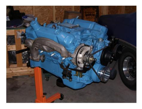
And finally the motivation, a 440 overhauled by R & R Speed Shop, with 9 to 1 compression and Comp Cams cam 268/268 duration and .454/.454 lift. The cam was selected for strong torque in the mid range and good drivability.
