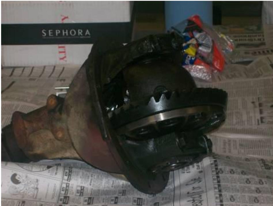
Next we measured the back lash on the gears to see if it falls within the factory tolerances. They did.
