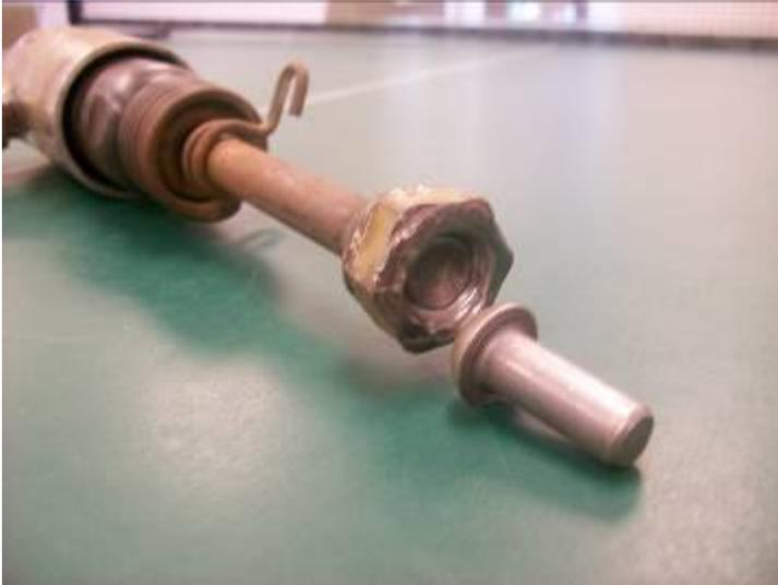
Nut welded to air hammer shaft. Perfect tool for the job.
